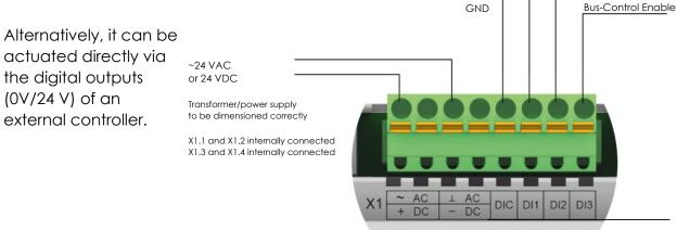
Optocoupler inputs with common GND
