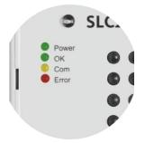
The unit has two damper position LEDs for each damper and an error LED. The fourth LED indicates the damper selected which can be tested directly via the unit. **Press both buttons** for more than 3 seconds to start an automatic search. As a result, SLC connections not being used will be deactivated and removed from the relay logic.
